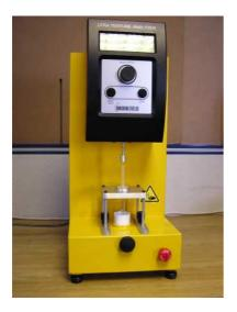
The test rig will quantify the force required to perform extrusion and extraction of an injectable solution using a syringe. The information is important for manufacturers in optimising the quality of the syringe as well as patient comfort and safety.
