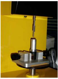
• Comparison of hardness of two different lipstick batches by penetration with a 2 mm needle probe- an adaptation of ASTM Standard method D 1321-95
